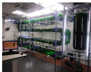
Microalgae cultivation in automated photo-bioreactor monitored by SCADA
