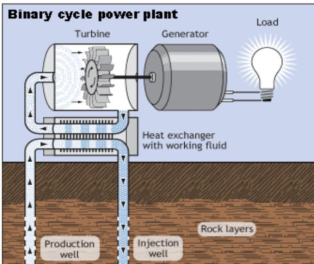
Binary cycle geothermal power plant
