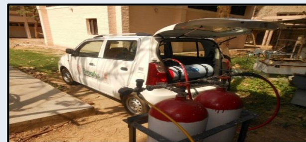
Enriched & bottled biogas dispensing system.
