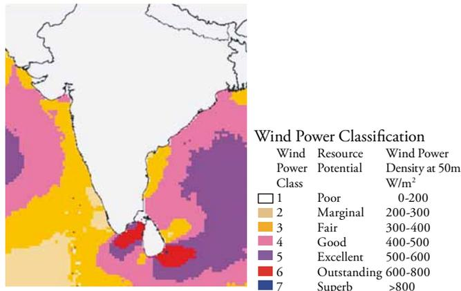
Fig 2. Wind density at 50 m height
