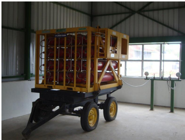
Cascade of 20 cylinders of 80 ltr. Capacity each at village - Talwada, Taluka - Trimbakeshwar, District - Nasik (Maharashtra)
