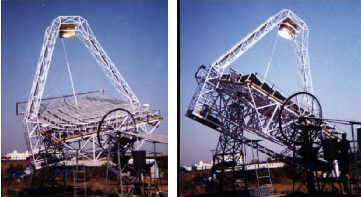
Figure 4 : ARUN30 - The concentrating solar collector of 30 m<sup>2</sup> area tested in December 2001 at Pune
