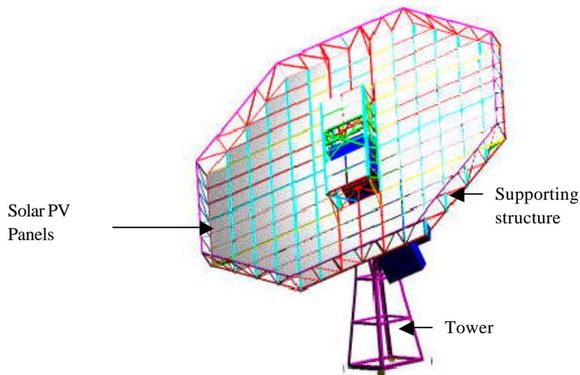
Figure 7 : Solar PV Panels on tracking structure for 30% more generation of energy
