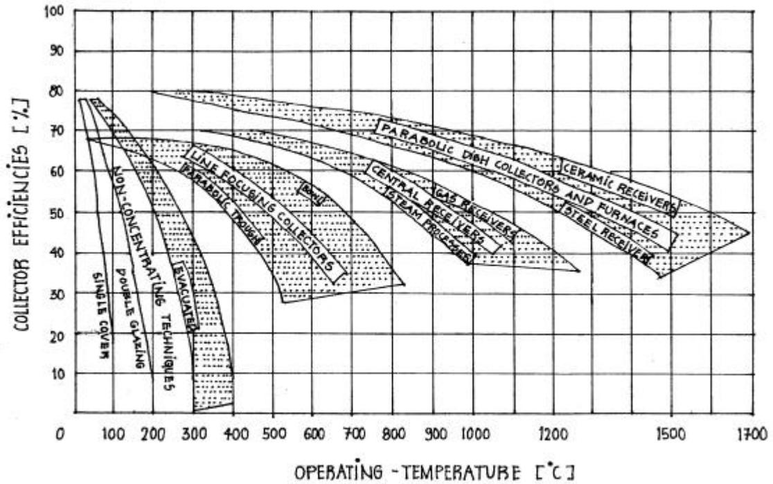
Figure 1 : Comparative efficiencies as function of temperature for different solar thermal technologies
