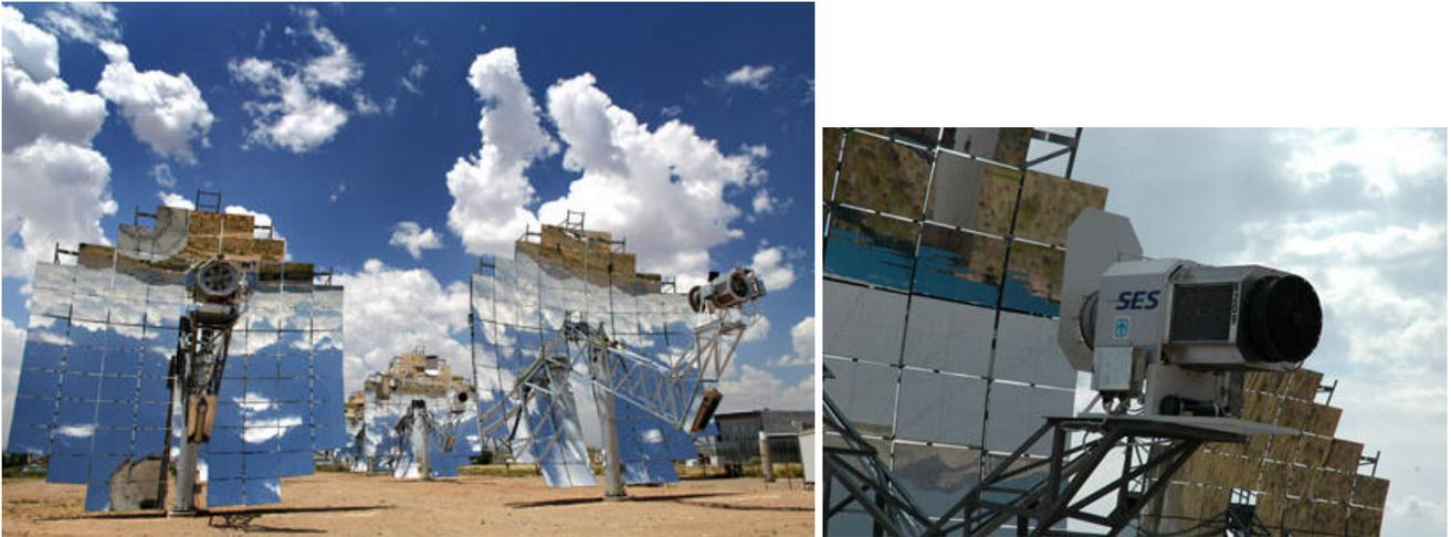
Figure 6 : Picture of a few of the 6 dishes tested at Sandia Lab with a close up of the Stirling engine at its focus
