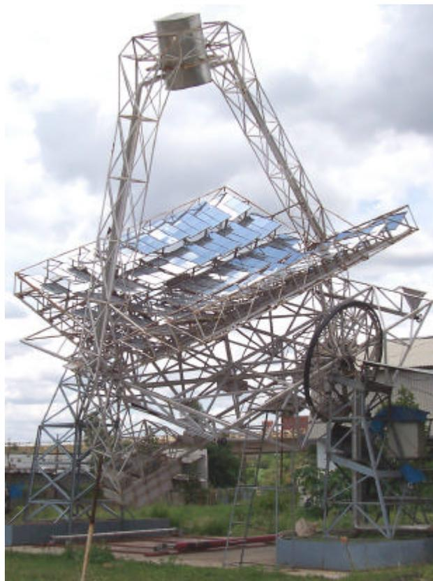
Figure 5 : ARUN™ : The Fresnel Paraboloid Concentrator with Point Focus tested at Pune in 2003
